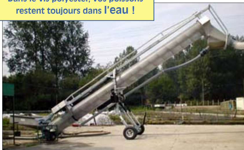
Série 85 vis Ø450mm long. 5m - option EPHP.
